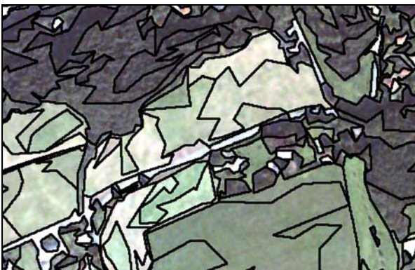
Figure 7. Segmentation result of the 'Minimum Entropy Approach'.
