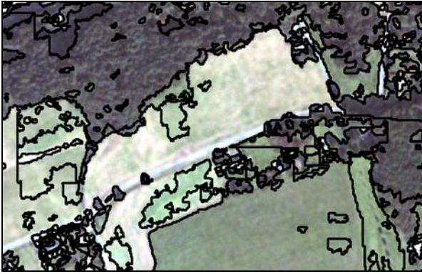
Figure 6. Segmentation result of the Erdas extension 'Image Segmentation'.
